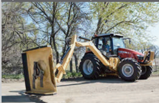
Triple Flail mowers available up to 22' wide.
