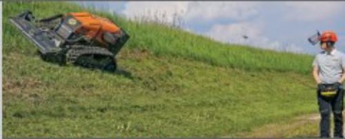
Energreen Robo Remote Controlled Steep Slope Mower
